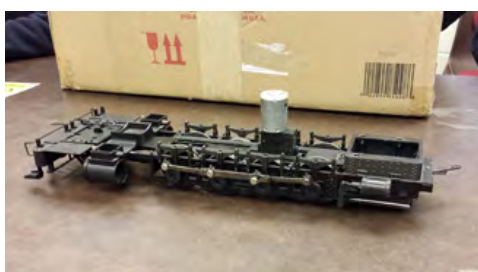
Alec Escolme: Frame and smoke box for Denver Rio Grand C25 Conversion for garden railway (45mm)
