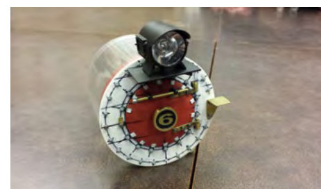
Alec Escolme: Frame and smoke box for Denver Rio Grand C25 Conversion for garden railway (45mm)
